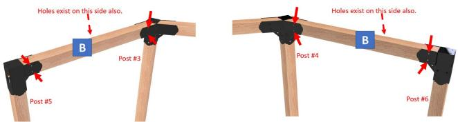
3. Drill 3/32" X 1-1/4" deep pilot holes at the center of 5/16" holes at both ends of the header and on both sides. Locate pilot holes at the center of each 5/16" hole. Perform this step for both "B" headers.
