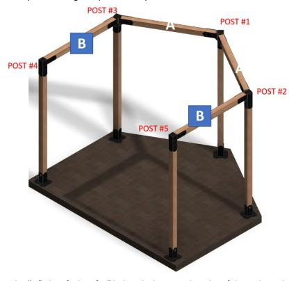
2. At both ends of header "B," identify the 5/16" holes which are on the sides of the U-channel in the elbow brackets. Holes exist on both inside and outside faces of the brackets.
