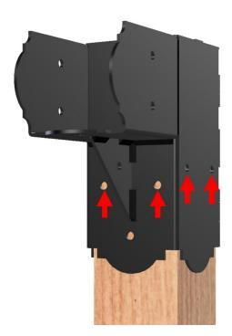
3. Drill 3/32" X 1-1/4" deep pilot holes at the center of four 5/16" Holes. Locate pilot holes at the center of each 5/16" hole.
