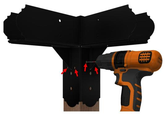
5. Drive one ¼ x 1-1/4" Lag Screw through each 5/16" hole into the pilot holes you drilled in step 4, using a 7/16" Socket and Rachet driver. Tighten down each screw.
