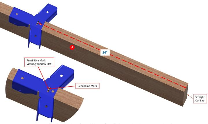
3. Position one cross tie bracket with the 24" pencil line mark inside the pencil mark viewing window slot. Center the pencil mark within the slot. The U-channels face downward, as shown in the images, above.
