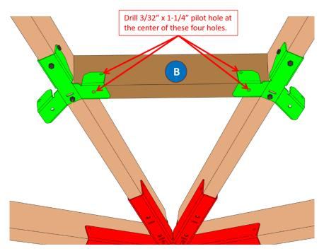
3. Drive one ¼" X 1-1/4" lag screw through the four pilot holes you drilled. Tighten the lag screws.
