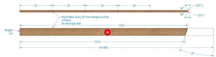
2. Make a pencil mark every 24" on the longer side of the rafter, starting at the straight cut end. The pencil marks must be on the longer side of the rafter member. This longer side will be the bottom surface once the rafter is mounted.
