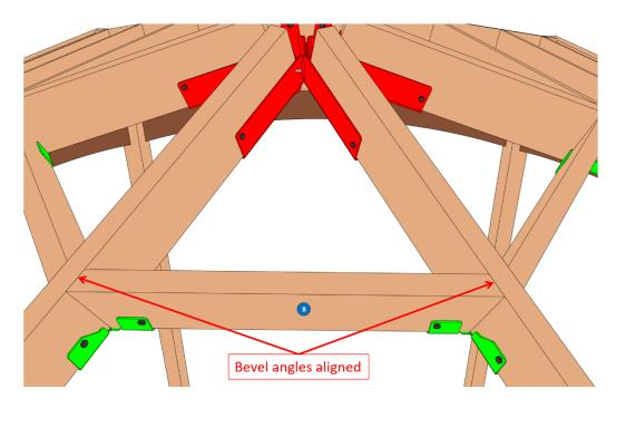
2. Identify two holes in each cross tie bracket, see below. Drill 3/32" x 1-1/4" pilot holes at the center of these four holes.
