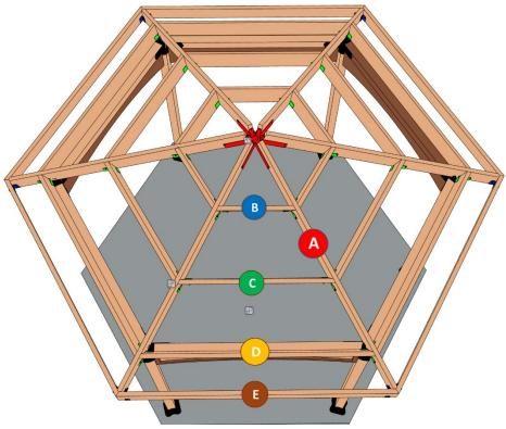
1. Lift and place one Beam B in the U-channels of adjacent cross tie brackets. Match the bevel angle in the cross tie beam ends with the tapers of the rafters. The cross tie beams will sit properly in one orientation only.
