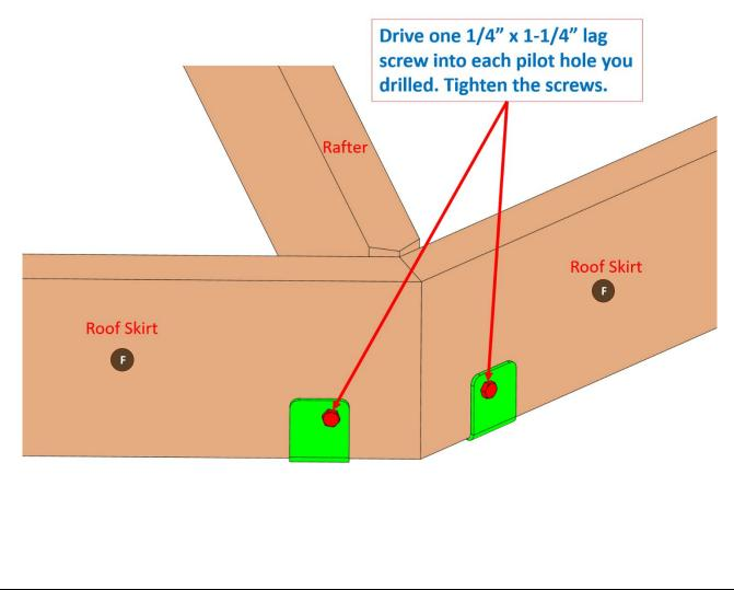
5. On the inside surface of the Roof Skirt member, identify two hole, as shown, below. Drill 3/32" x 1-1/4" pilot holes in the center of the these two holes. Note: Extend the drill bit out as far as possible in the drill gun. Drill holes upward at a slignt angle.
