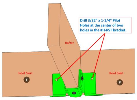
6. Drive one ¼" x 1-1/4" lag screw into each pilot hole you drill in step 5. Tighten the lag screws.
