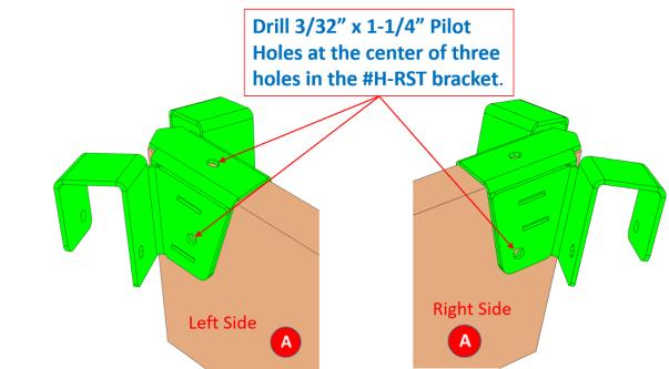
4. Drive  $\frac{1}{4}$  x 1-1/4" lag screws into the three pilot holes you drilled in step 3.
