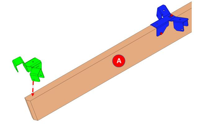
2. Position the #H-RST bracket with its V-shaped end aligned with the V-shaped edges of the bevel cuts.
