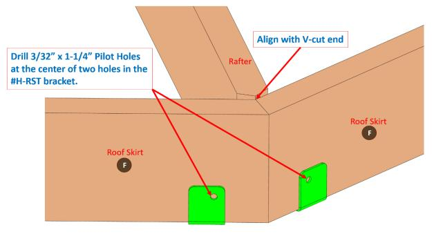
4. Drive one <sup>1</sup>/<sub>4</sub>" x 1-1/4" lag screw into each pilot hole you drill in step 3. Tighten the lag screws.
