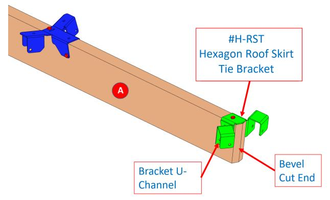
1. Place one #H-RST bracket on the bevel cut end of a rafter member, as shown.
