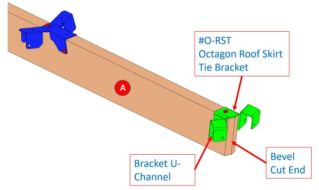
1. Place one #O-RST bracket on the bevel cut end of a rafter member, as shown.
