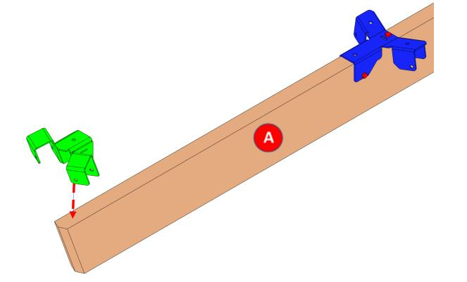
2. Position the #O-RST bracket with its V-shaped end aligned with the V-shaped edges of the bevel cuts.
