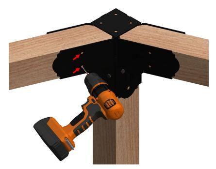
4. Drive one 3/8" X 2"" Lag Screw through each 7/16" hole into the pilot holes you drilled in step 8, using a 9/16" Socket and Rachet driver. Tighten down each screw. Repeat for opposite side of the U-channel and the opposite end of the header.
