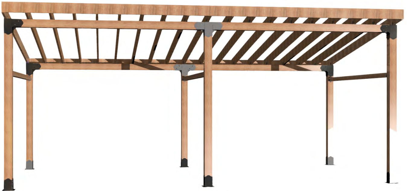
Figure 1: 24 ft. x 12 ft. Concrete Mounted Lean-To Customized and prepared for: Emil Thomas
